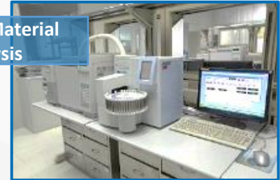
ATD-GC/MS Range: 1.5~1050 amu Resolution : 2 nano gram
