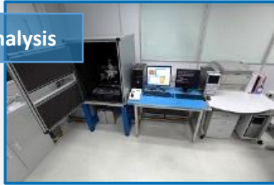
AFM Resolution : 0.1 nm
