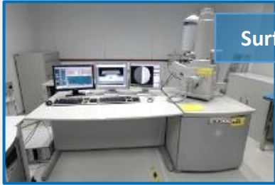
FE-SEM/EDX Mag: 80x ~ 300,000x Resolution : 3.5 nm
