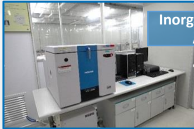
XRF Zn, Ni, Cr, Cu, Ag, Au, Sn Area : > 1 mm 2 Thickness : 0.25~65um
